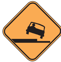
Pavement Drop Off
